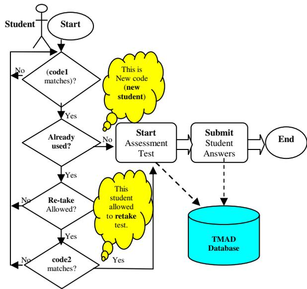
Figure 7. Test code Algorithm for (Re) Take Test
